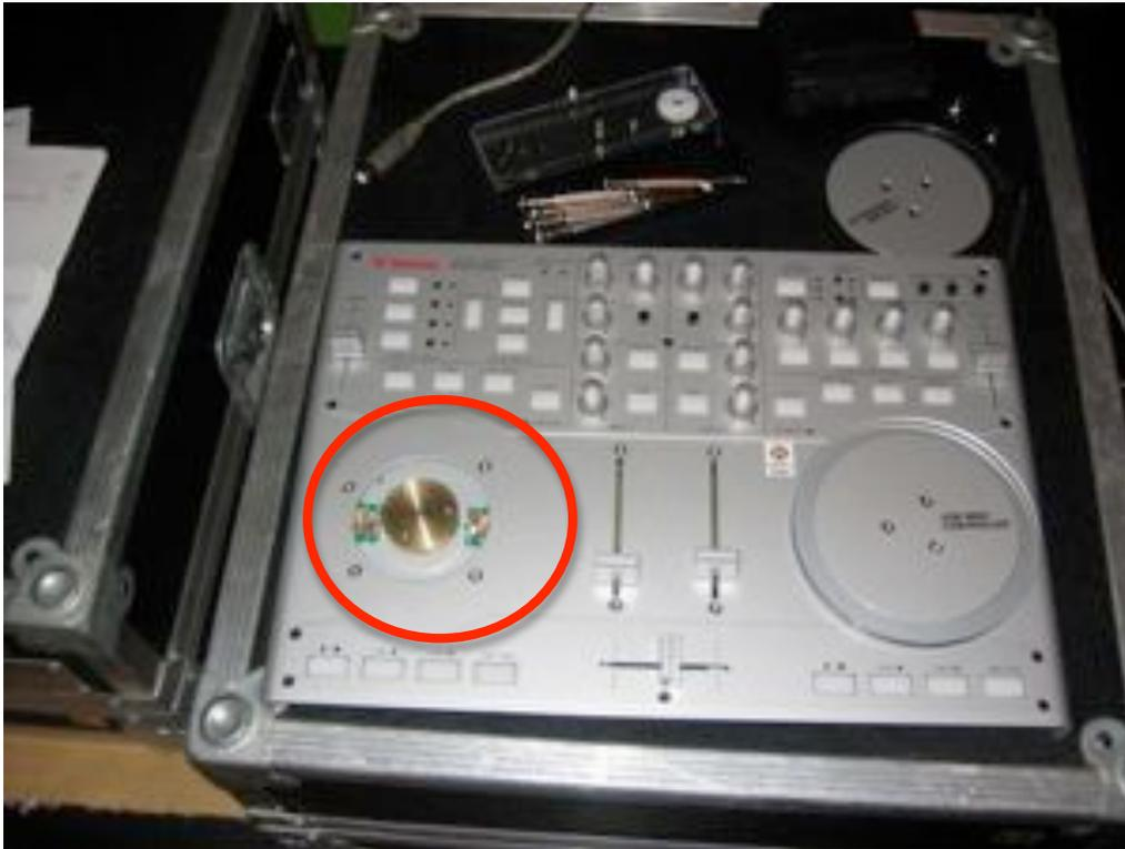
6) Remove the four screws holding the encoder in place. Note that these screws have absolutely no bearing on how well the VCI rotates, they are just to hold the encoder in place.
