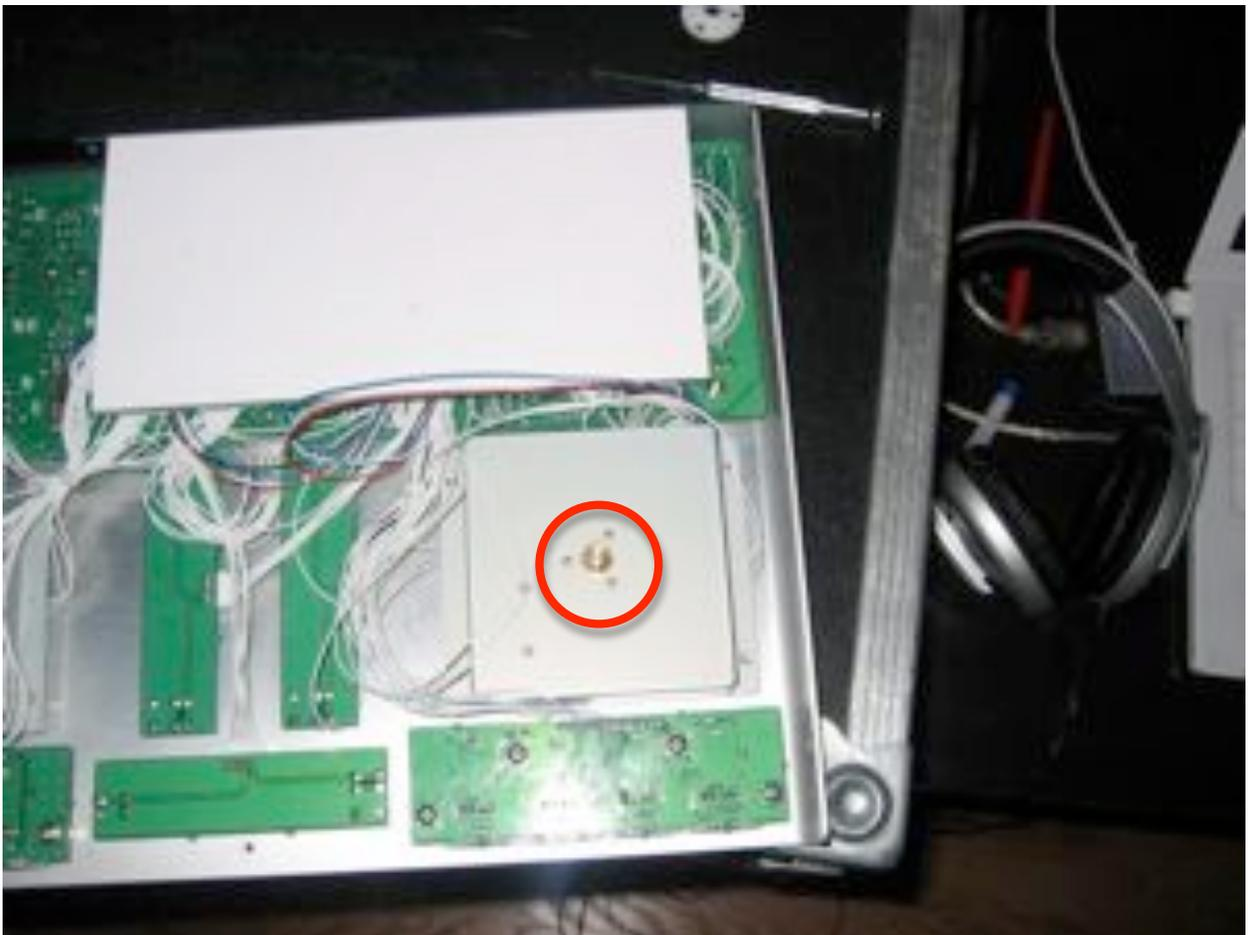
Two warnings though! First, **only use a single drop of lubricant** – seriously. A single drop is more than enough. Secondly, try to make sure the lubricant is electrically conductive. The lubricant can cause the contact resistance (the electrical contact
